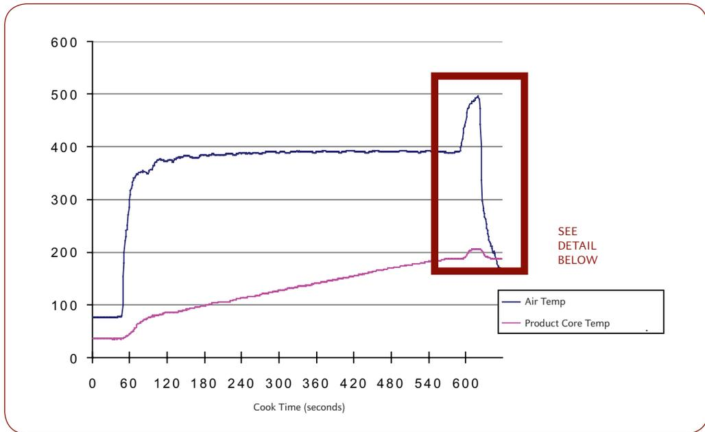
The effect of zone separation is clearly demarcated in the above graph. The air temperature (in blue) in the main stack is maintained at 390°F (199°C) even very close to the impingement module. The sharp spike in air temperature is experienced by the product only upon entering the impingement module.
