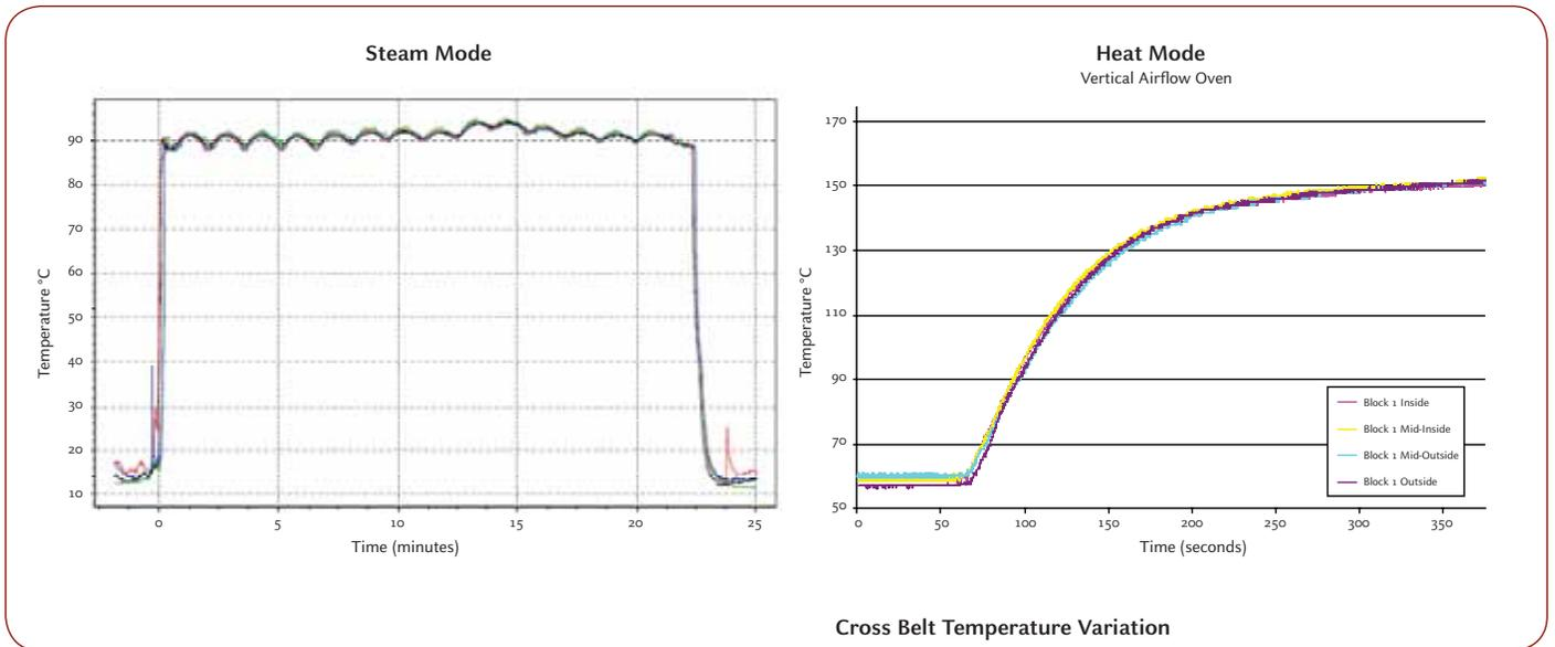
In a Stein GYRoCOMPACT II Oven, cross-belt air temperature variations during both steaming and convection cooking are less than  $\pm 2^{\circ}\text{F}$  ( $1^{\circ}\text{C}$ ).
