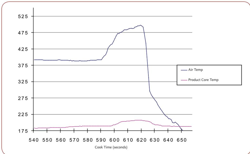
True impingement finishing in the Stein GYRoCOMPACT II Oven provides an isolated, controllable cooking environment that combines high-velocity convection of up to 4,000 ft/minute (20 m/sec) with temperatures up to 540° (282°C). This coupled with a temperature differential of up to 200°F (112°C) between the cooking environments in the spiral stack and the impingement module can drive the core temperature of the product the final 5-10°F (3-6°C) in as little as 30 seconds.
